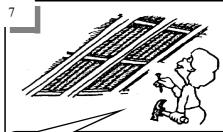
INSERT CEILING FRAME AND FIX WITH SCREWS PROVIDED. PLASTIC LUGS ARE PLACED ON TOP SIDE OF CEILING. FIX SCREWS THROUGH HOLES IN CEILING FRAME
