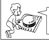
USING THE FOUR "GREY" SCREWS PROVIDED, SCREW THE ACRYLIC DOME TO THE BLACK ROOF FRAME. THE DOME WILL HAVE PREDRILLED HOLES IN ITS BASE.
