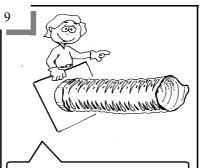
ALLOW SUFFICIENT LENGTH OF FLEXI-TUBE TO REACH FROM ROOF TO CEILING (REMEMBER TO ALLOW FOR BENDS IN FLEXI-TUBE). TAPE THE BOTTOM STAINLESS STEEL RING TO THE FLEXI-TUBE.
