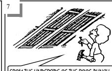
FROM THE UNDERSIDE OF THE ROOF PUNCH OR DRILL A HOLE AT THE CENTRE OF WHERE THE SKYLIGHT DOME IS TO BE LOCATED THE HOLE IS TO BE ON THE DIP (LOW POINT) OF A CORRUGATION.
