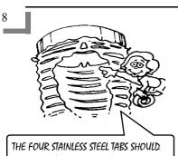
BE BENT OUTWARDS THROUGH THE FLEXI-TUBE THEN BEND INTO HOOK SHAPE TO HOLD THE WIRE .... BE SURE TO COVER THE TABS WHEN TAPING
