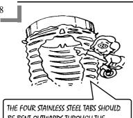
BE BENT OUTWARDS THROUGH THE FLEXI-TUBE THEN BEND INTO HOOK SHAPE TO HOLD THE WIRE .... BE SURE TO COVER THE TABS WHEN TAPING
